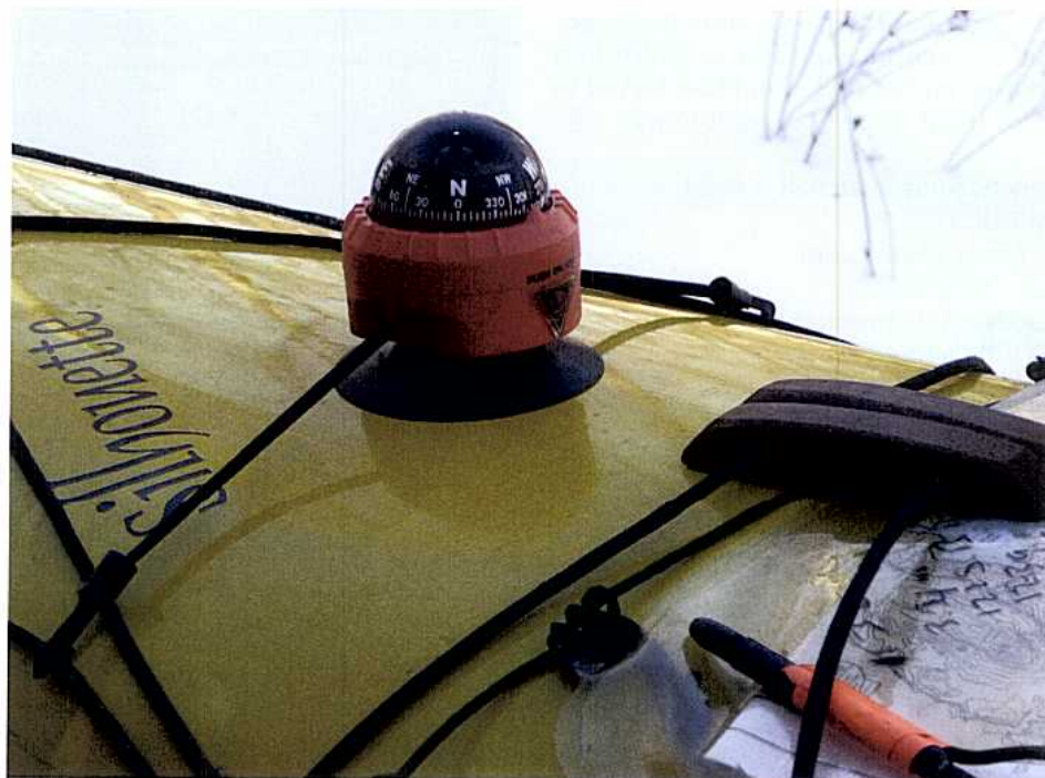
The compass is secured to the deck by a rubber suction cup clipped into the deck lines with a pair of bungees and hooks. Photo: Ben Fuller.
